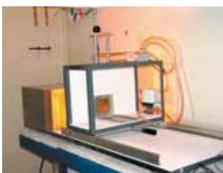
Radiant panel test: meet de neiging tot vlamverspreiding - vloerbekleding.
